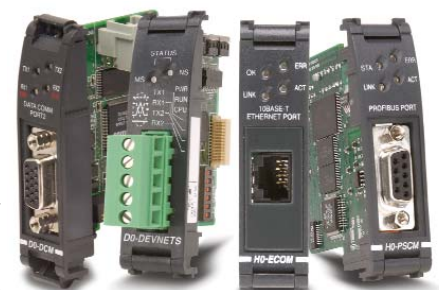
Modbus DeviceNet Ethernet PROFIBUS (Modbus TCP)
