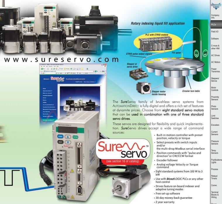
For configuration, tuning and diagnostics, use the drive's integrated keypad/display or take advantage of the free SureServo Pro™ PC-based software. Tune the system easily with adaptive auto-tuning selections or manual mode. Adapt to diverse applications with configurable I/O, including 8 digital inputs, 5 digital outputs, 2 analog monitors and a scalable encoder output.
