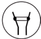
IEC 60947-5-1 Mechanically linked contacts
