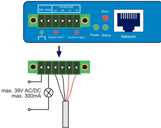
The output of the Web-Thermograph Relay is switched internally using a relay contact (normally open). The consumer is connected to the screw terminals 1 and 2. The maximum switchable DC or AC voltage is 39V, with a maximum current flow of 300mA.
