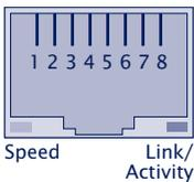
The network connection is galvanically isolated with respect to the supply voltage as well as the serial interface(s) for at least  $1,5\text{kV}_{\text{rms}}$ .
