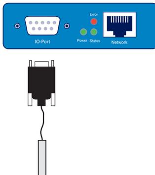
Plug the sensor included in the scope of delivery into the 9-pin IO terminal on the unit.
