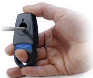
DN-CST Precision Stripping Tool [squeeze, insert cable, rotate, & remove]
