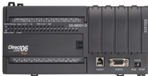
DO-06DD1-D $251.00 DC in/DC out/DC supply
