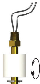
Figure 1: Vertical (Top) Mount Switch Operation
