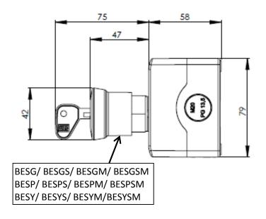
10. Mounting emergency stop push button on panel with special NC contact block monitored.
