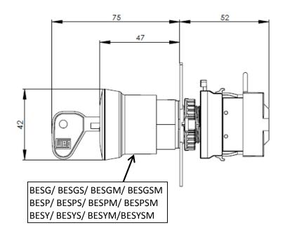
12. Mounting emergency stop push button on control station with NC contact monitored by an ordinary NO contact.
