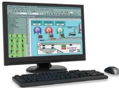
In a PC-based control system, a standard operating system such as Windows NT supports HMI and control software running on a PC platform, either a readily available commercial model or an industrially hardened unit. PC architecture allows the system to seamlessly support a variety of third-party I/O, specialty motion and vision systems, and field networks.
